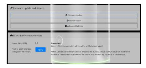
Set the tick-mark for "Enable direct LAN" and press Apply.
